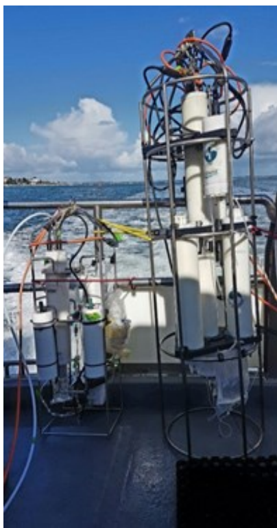
Figure 10: (Left) TMSM and (right) Integrated system incorporating one TMSM, CSM, ASM and CTD.
