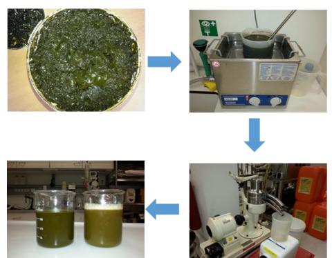
**Figure 7**. Separation of amino acids by laboratory centrifuge at biomass: water ratio of 1:9.
