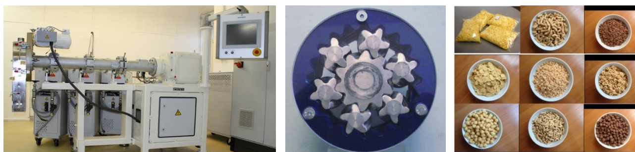
Figure 22. Planetary roller extruder (left); central spindle (centre); extruded minor cereals (right)
