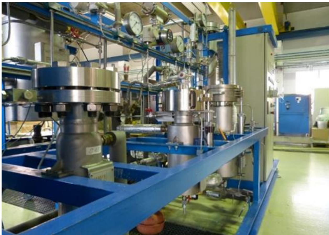
Fig. 4. 5L/1000bar supercritical CO 2 extraction unit in Natex laboratory
