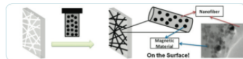
Fig. 1. Last step in the process of synthesizing the adsorbent consisting of PAN-SPION nanofiber. SPION is represented by black circles and PAN is represented by white strands. SPION is placed on the surface of PAN.
