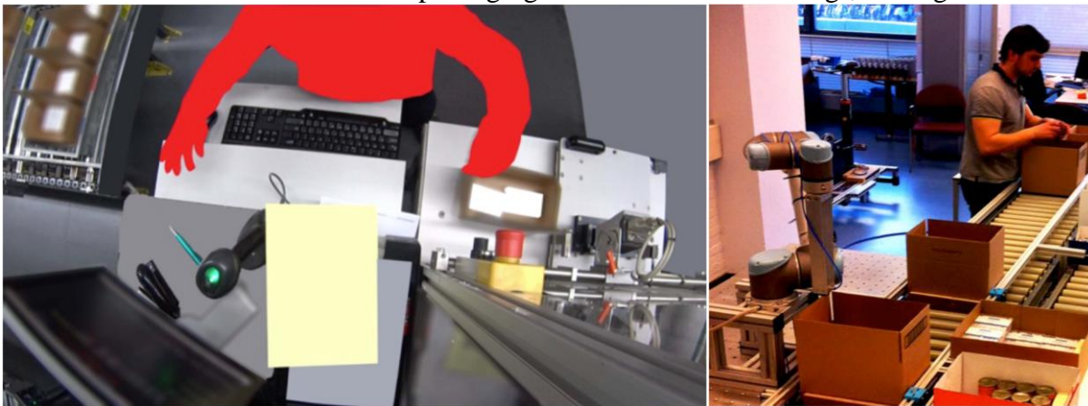
Figure 4: Left: top view of a test setup for a machine tending task, to study the physical and cognitive (information) activities of a human operator. Right: realistic test setup to analyze human-robot interaction (both physical and cognitive) during collaborative box packing.
