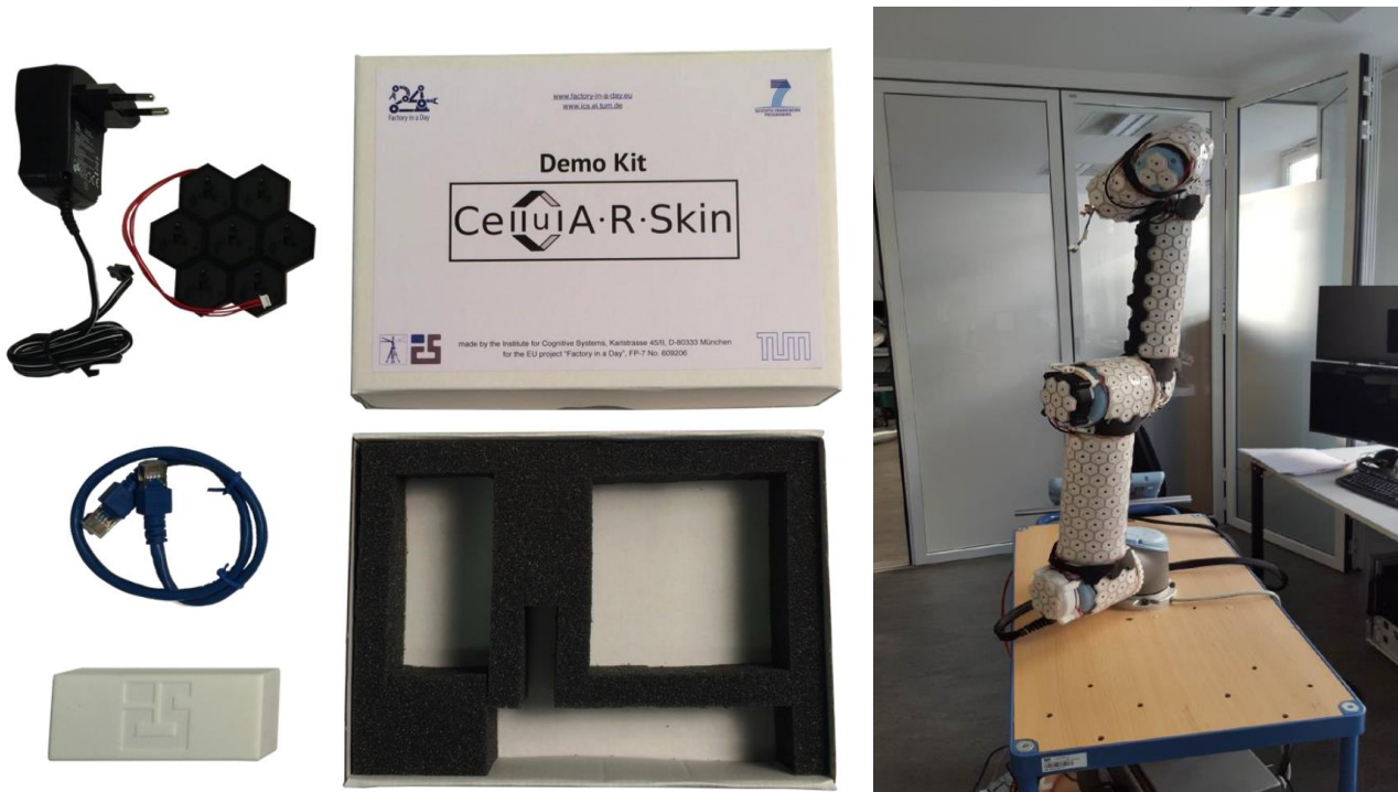
Figure 14: Left and middle: prototype skin distributed at month 6. Right: Fully skin-covered robot arm.
