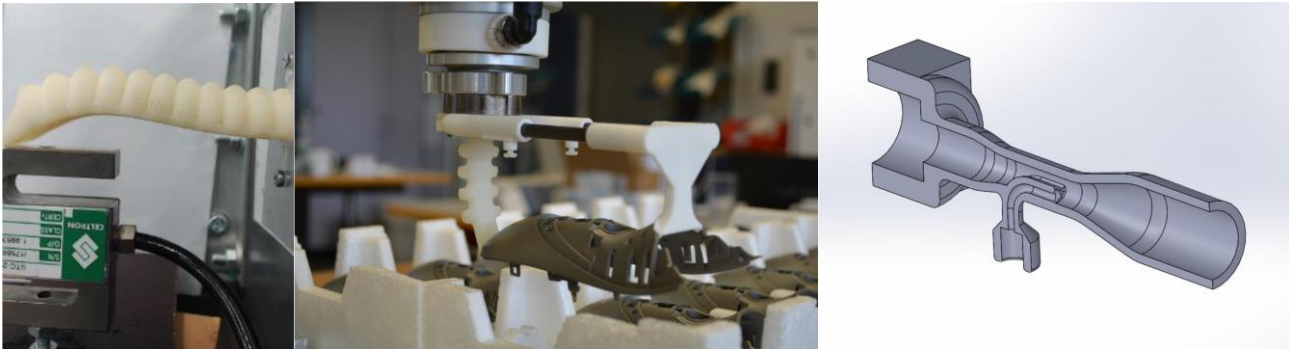
Figure 10: Left: bellows finger. Middle: Gripper for Philips case. Right: design for Venturi Finger.
