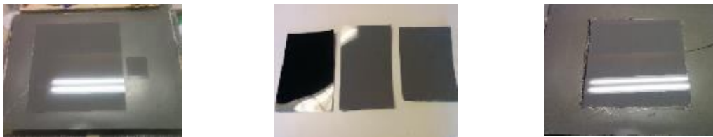
Figure 17. Different laminates obtained with Class A surface – tests for mould construction.
