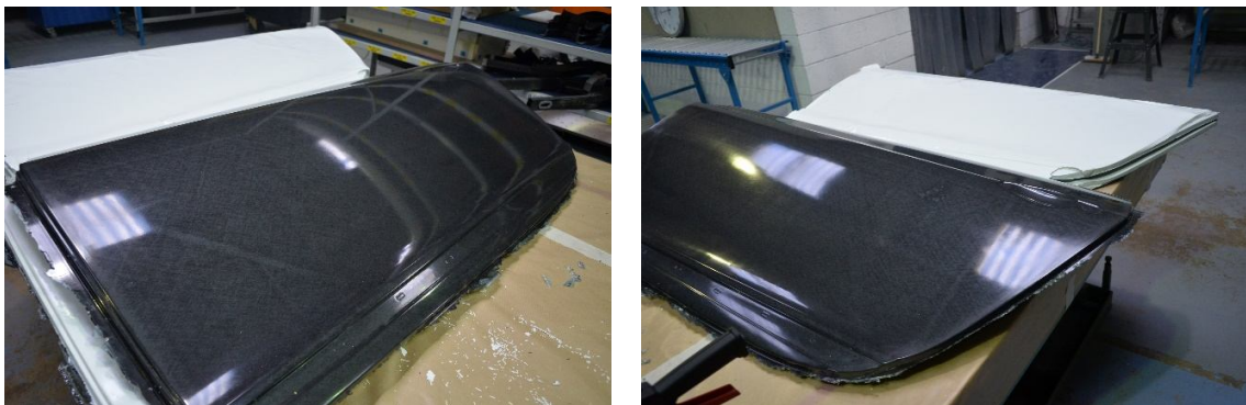
Figure 24. Door skin Black (conductive) and door skin White (non-conductive)
