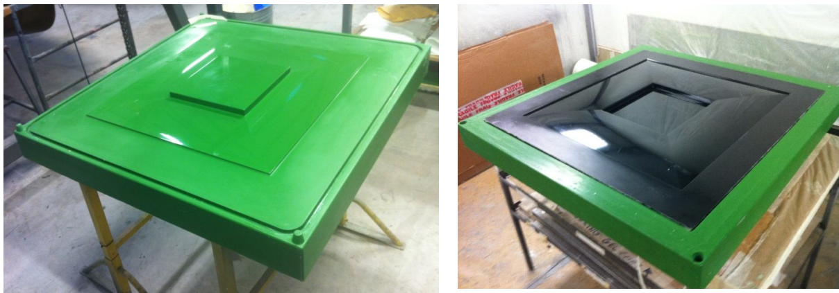
Figure 13. WP4 electrically heated mould.
