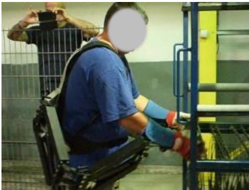
Figure 27 Lifting wiper curtains with the passive arm module
