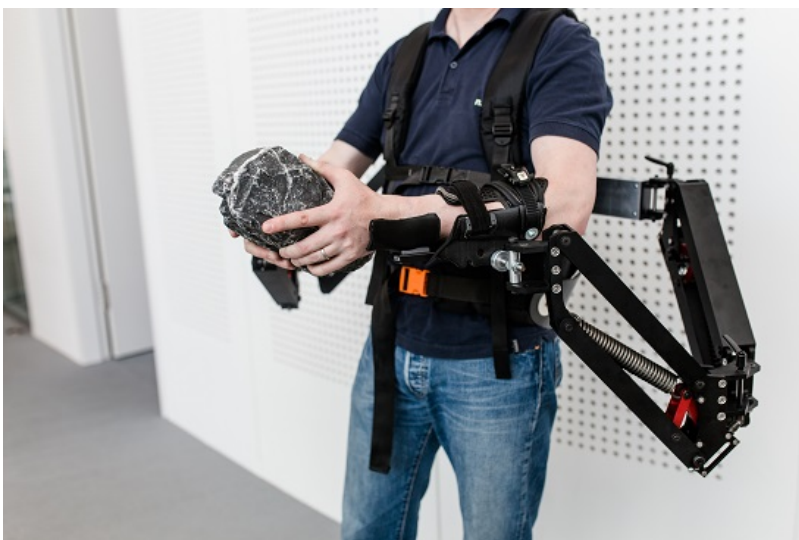
Figure 6: Passive parallelogram arm module (final prototype)
