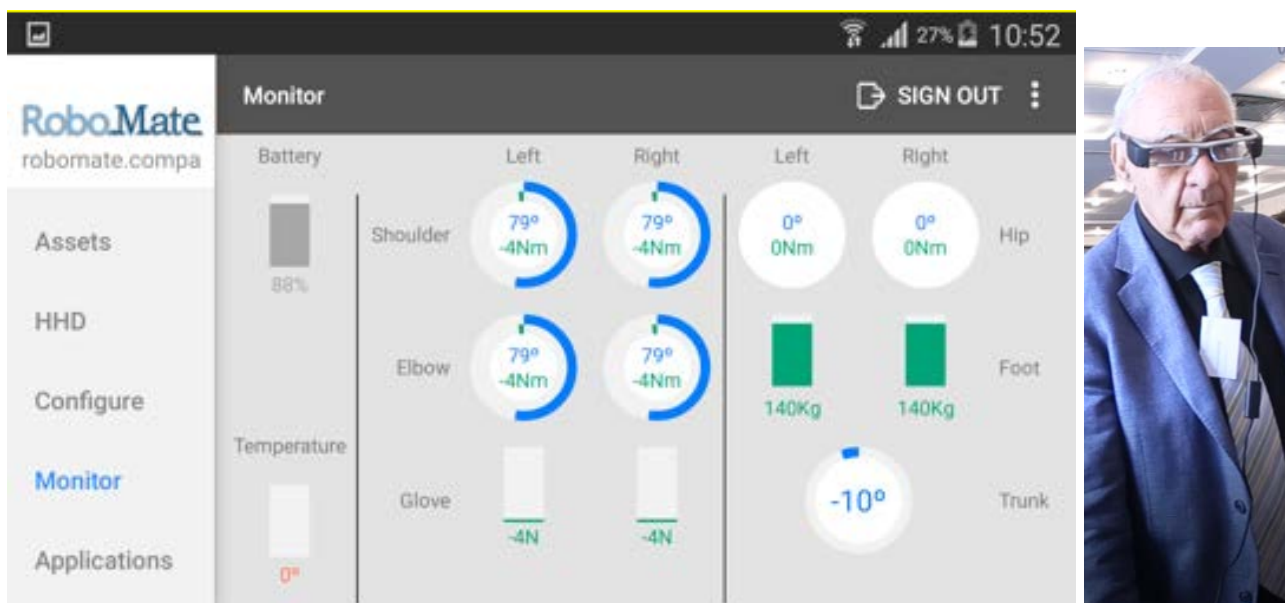
Figure 12: Human machine interface of the handheld device (left) and the smart glasses in use (right).
