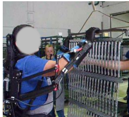
Figure 28 Lifting wiper curtains with the active arm module
