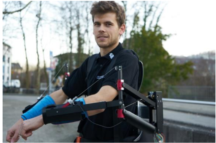
Figure 8: Active parallelogram arm module (final prototype)
