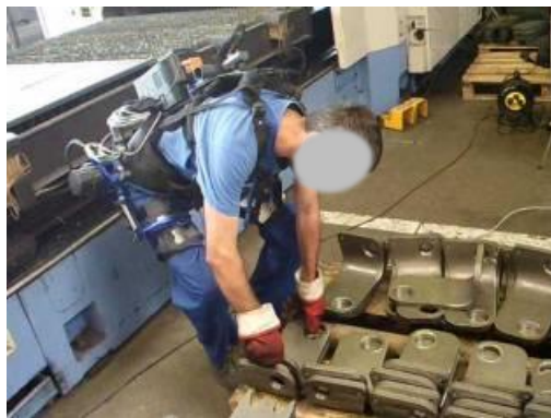
Figure 29 Handling of metal parts with the trunk module
