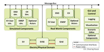
The figure below depicts how the different partners laboratories have implemented respective parts of the architecture, stating the current testing capabilities of the COTEVOS consortium utilizing a depiction of the 3rd layer of the COTEVOS common reference architecture.
