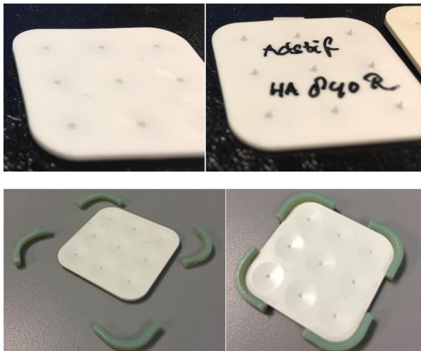
Figure 13: Actual microneedle array and external features to facilitate alignment.
