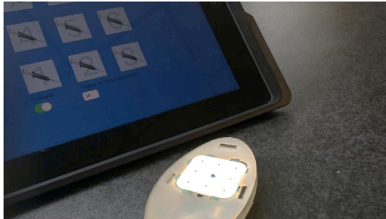
Figure 1 – Prototype of microneedle drug injector, to be miniaturized during the project. (source: Crospon)
