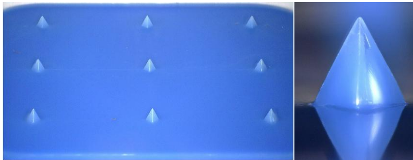
Figure 23 – Hollow microneedles made on plastic by injection moulding
