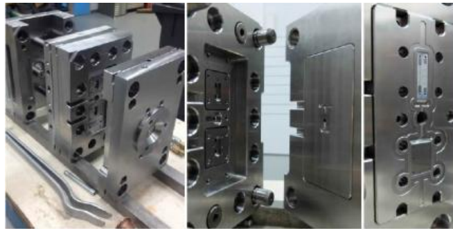
Figure 20 - Manufactured injection moulding tool and mould inserts before replication experiments.
