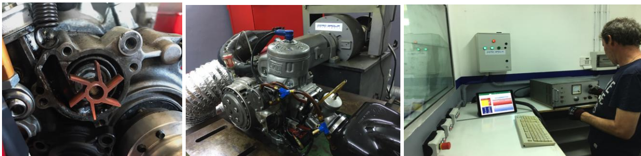
Fig. 23: Test bench validation of MicroFAST cooling turbine
