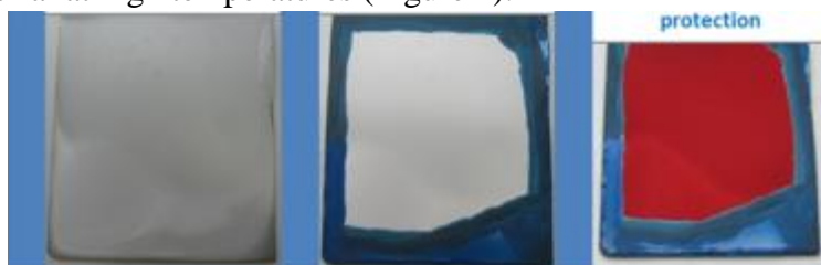
Figure 3: Top-coats tested on aluminium deposits from ionic liquids based electrolyte
