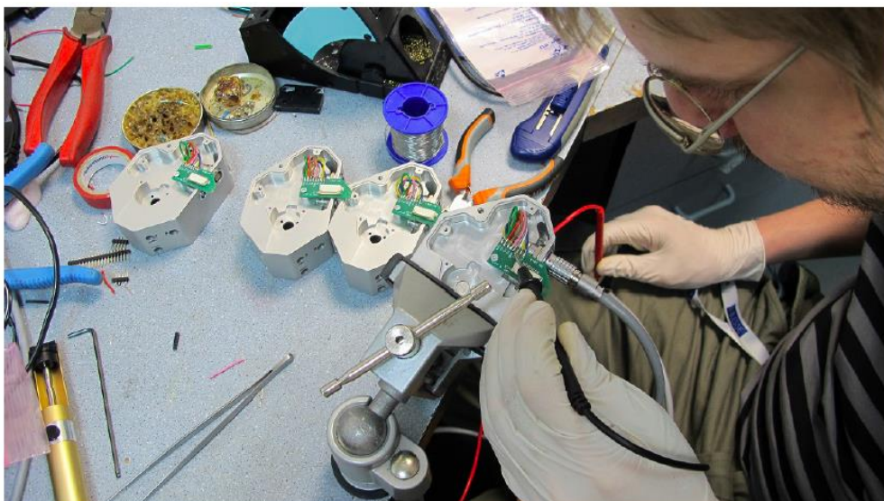
Fig. 3.3: Construction of the autocorrelator prototypes at UWAR.
