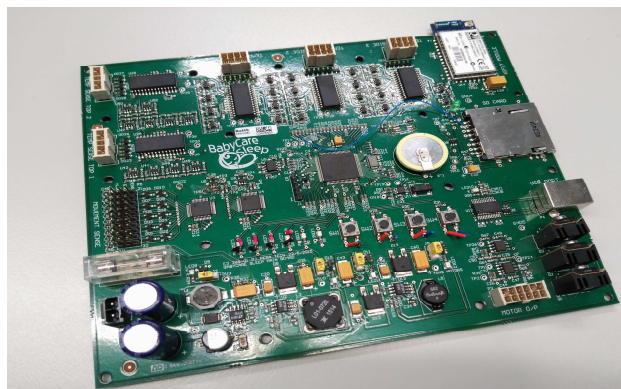
Figura 4. Electronic board for the control of the biosensing textiles of the mattress and the communication.
