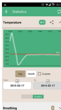
Figure 11. The app can receive information from the mattress and can display charts of the evolution of the information. The example picture shows a chart with the evolution of the temperature (with sham data).
