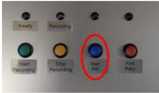
Figure 9. The button to force the set-up mode in the hardware prototype of the mattress.
