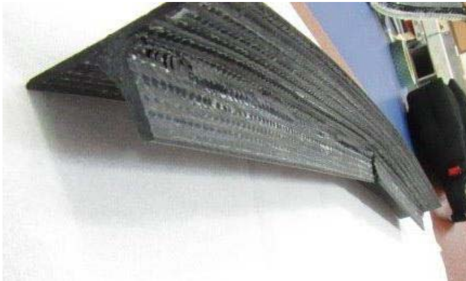
Figure 25. Section forming test with noticeable foot curvature and blade failure.
