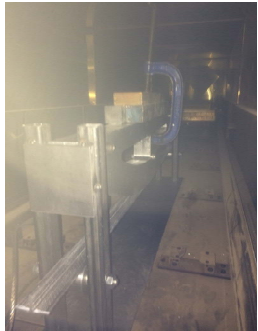
Figure 36. Positioning of stage 1 (semi-cured) profile under the forming tool (supported by the frame, left) for stage 2 processing. The frame is placed in an oven (right) to introduce the bending to the profile
