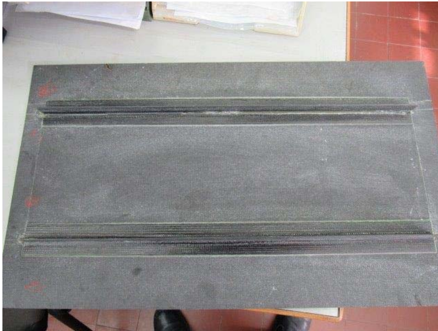
Figure 38. Co-bonded infused panel (stage 1 stringers bonded and cured on a composite panel at stage 2') processed at IAI
