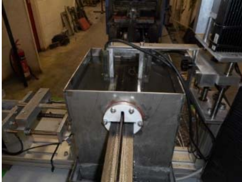
Figure 23. First profile exiting the water tank of the on-line QA system through the flange. Tight wiper ensures negligible water leakage and running on the surface.
