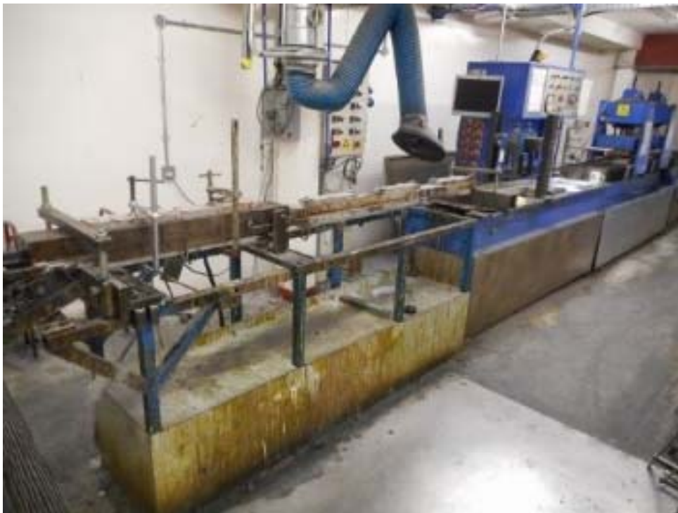
Figure 18. Set-up of the PUL-AERO pultrusion line for the installation of the new systems.
