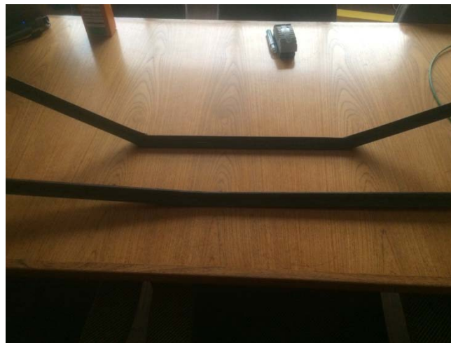
Figure 37. Stage 1 stringers subjected to bending during stage 2 processing at Exel
