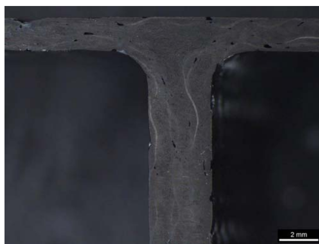
Figure 31. Microscopy on a section of semi-cured profile produced at the pultrusion line at Exel showing adequate quality of composite given a new resin material and injection system.
