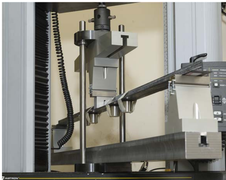
Figure 39. Details of the three-point bending test configuration for a semi-cured stringer of 1.1 m length
