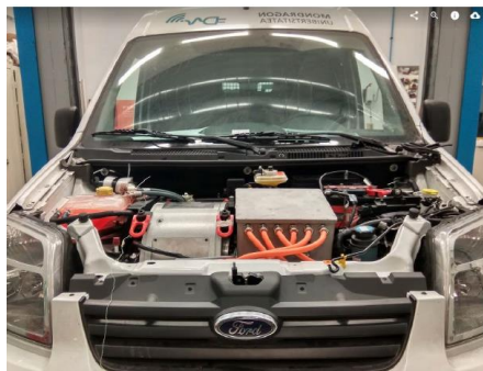
Figure 22. Full assembly of the new VENUS powertrain in operating condition.
