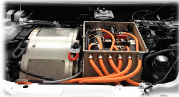
Figure 24. Motor and inverter integration finished (cover of the inverter is removed for display purposes).
