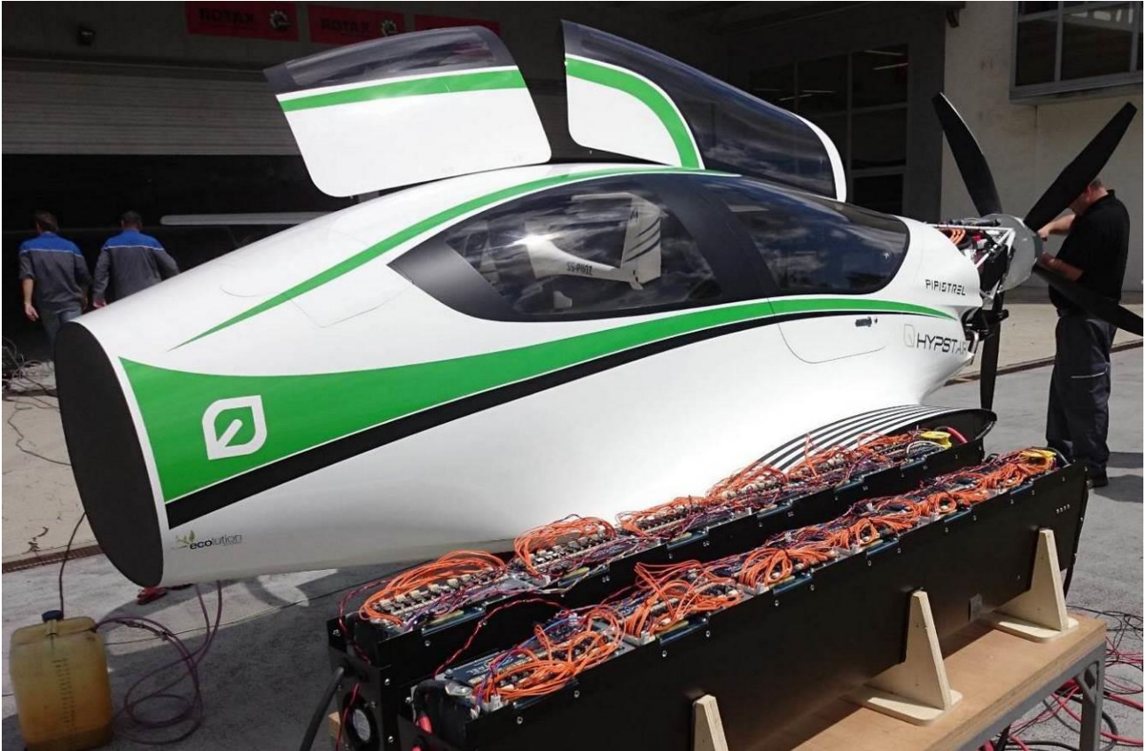
Figure 17 The HYPSTAIR propulsion battery developed by Pipistrel
