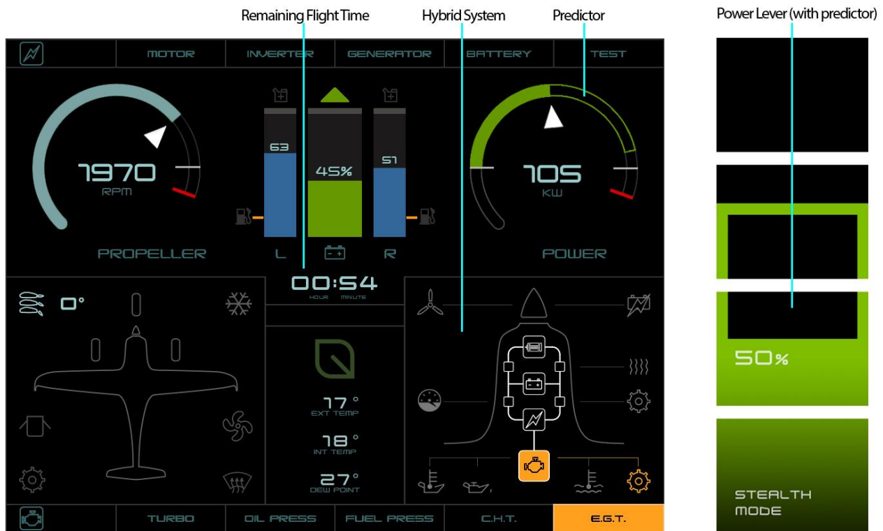
Figure 11: HMI design and power lever by MB Vision
