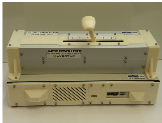
Figure 10: HYPSTAIR experimental prototype of the haptic power lever by University of Maribor
