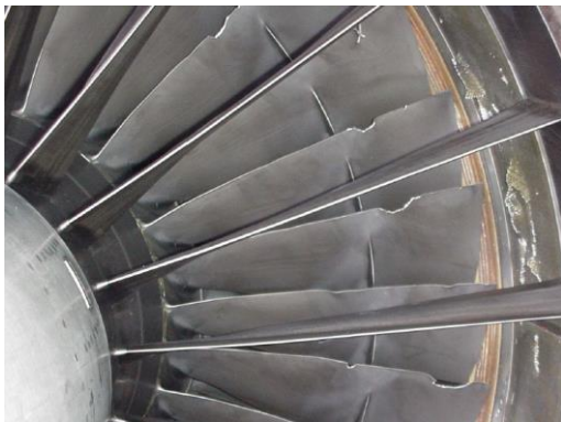
Figure 3: Rotor blades damaged by ice debris
