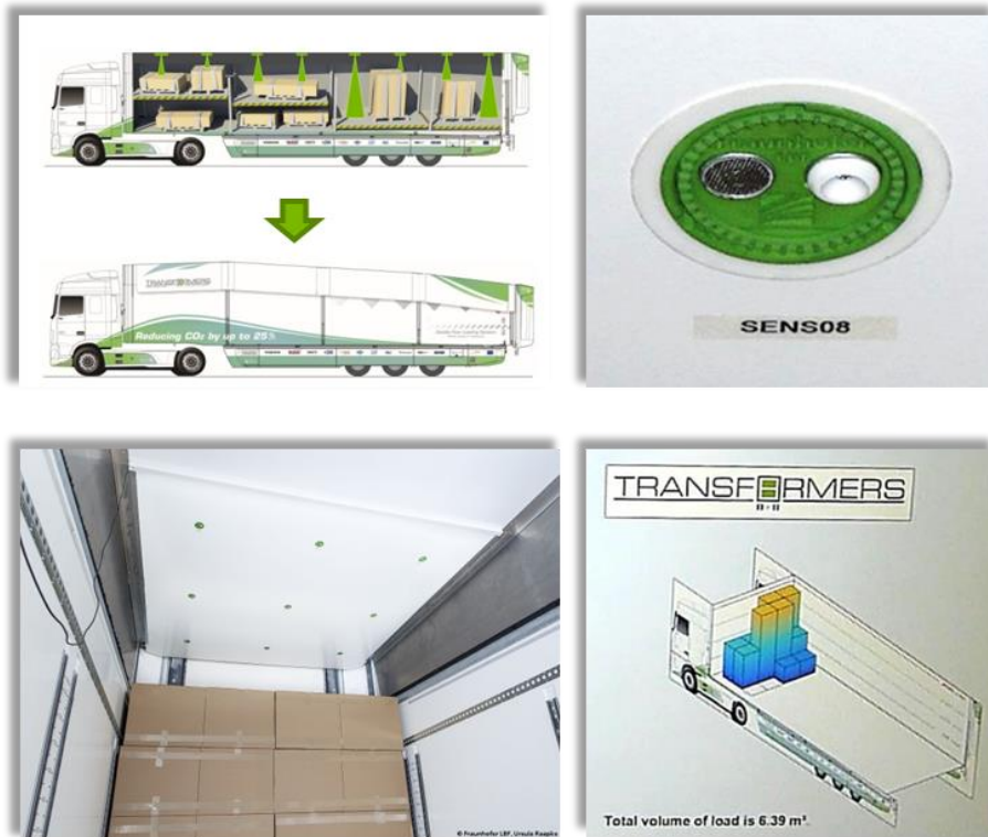
Figure 2-17: Load Optimisation Trailer: Load Volume Indicator System
