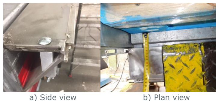
Figure 2-14: Load Optimisation Trailer: Collapsible Docking Plate Support
