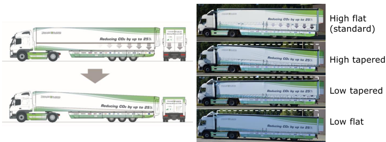
Figure 2-11: Energy Efficiency Combination Alternative Roof Positions
