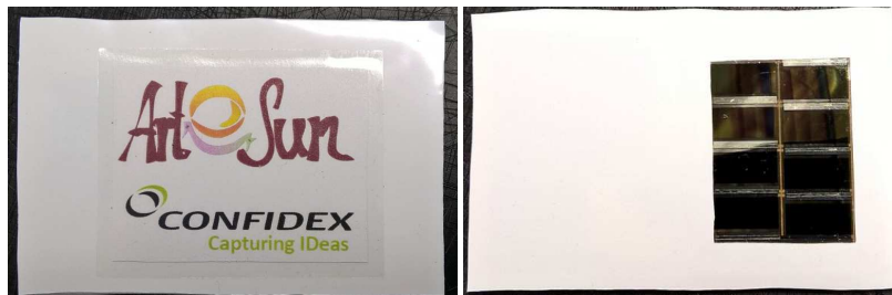
Figure 14 RFID-OPV device prototype with the label dimensions of 59 mm (W) x 90 mm (L) x 3 mm (T).
