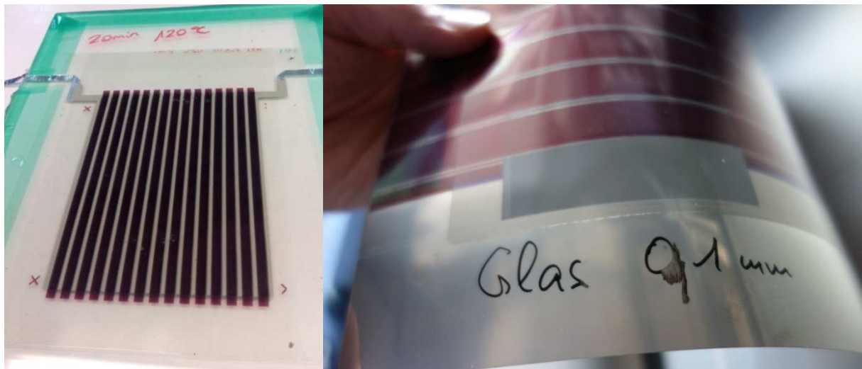
Figure 13 Photos of the large area Demonstrators, a plastic-film based module laminated into a BIPV façade element and a 30cm x 40cm large module processed onto a PV-barrier backsheet and encapsulated with 0.1mm thin willow glass.
