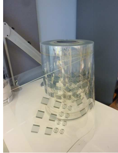
Figure 5 Novel ITO-free alternative electrodes based on silver grids and highly conducting PEDOT roll-to-roll printed onto PET flexible substrates.
