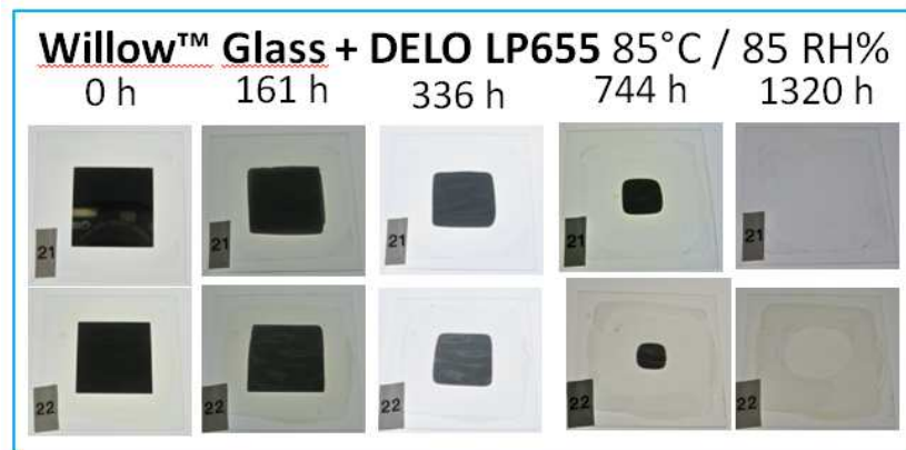
Figure 10 Result of the Ca test which clearly shows that main degradation channel is diffusion from the edges through the adhesive or at the adhesive/substrate interface.
