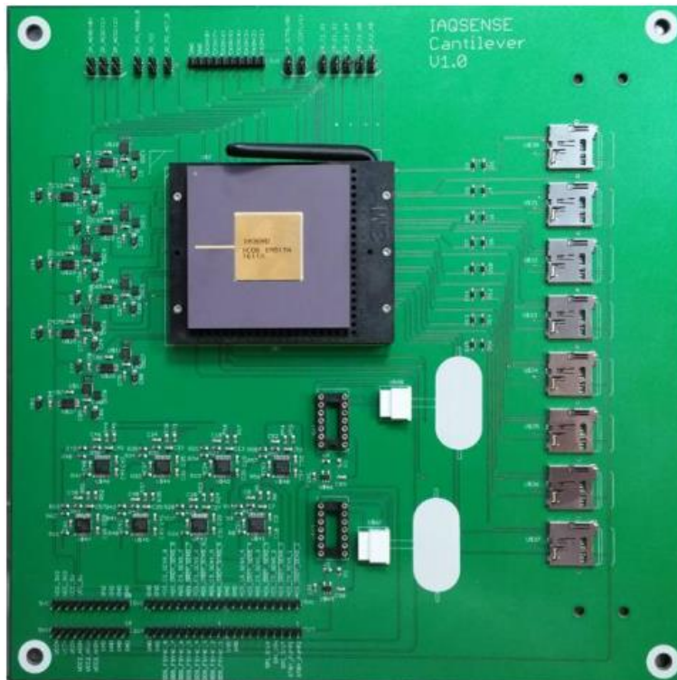
Figure 4 ASIC based (IM309D) 8-Cantilever board plus 2 optional piezo pumps for inject/purge pattern
