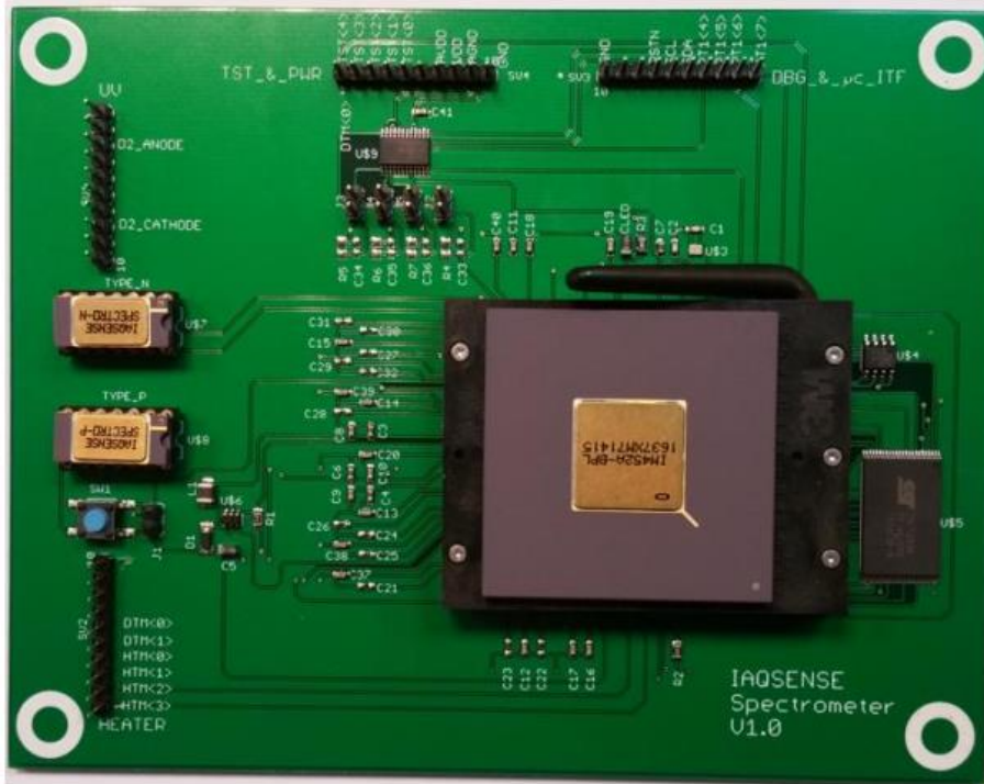
Figure 5 MOSFET spectrometer on chip demo board design by EELEO
