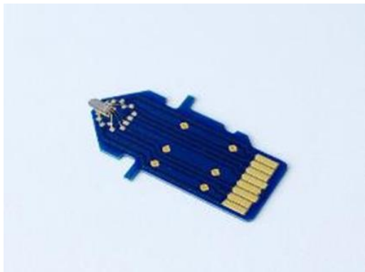
Figure 3 Cantilever bonded on a custom PCB holder (on the left) and cantilever bonded in standard TO12 package (on the right).
