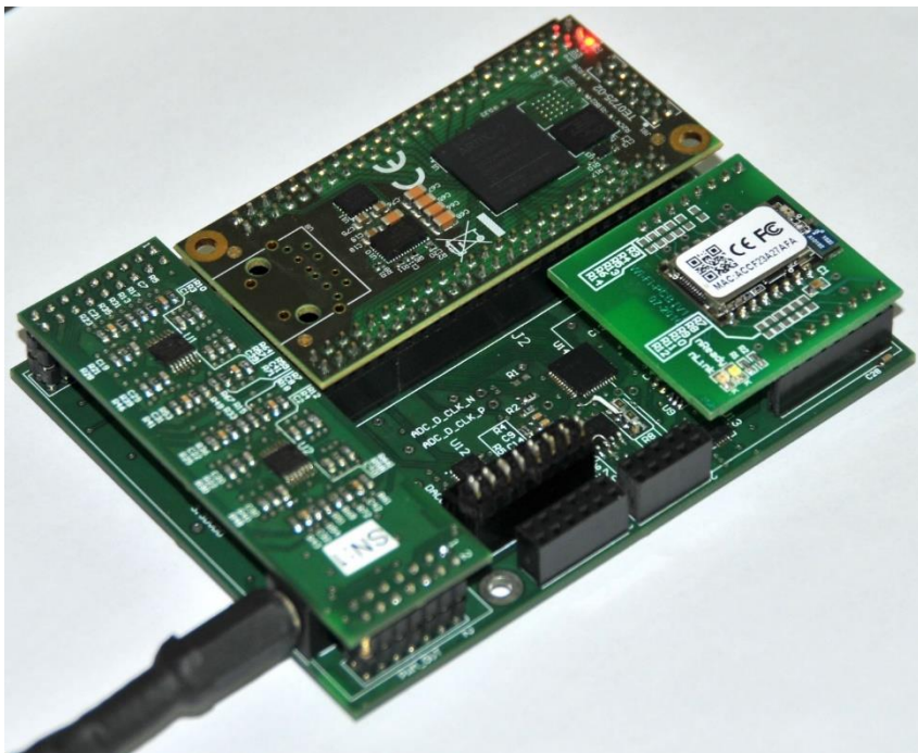
Dedicated Board with lock-in amplifier for acquisition of a 8-Cantilever network, using MSP432 DSP
