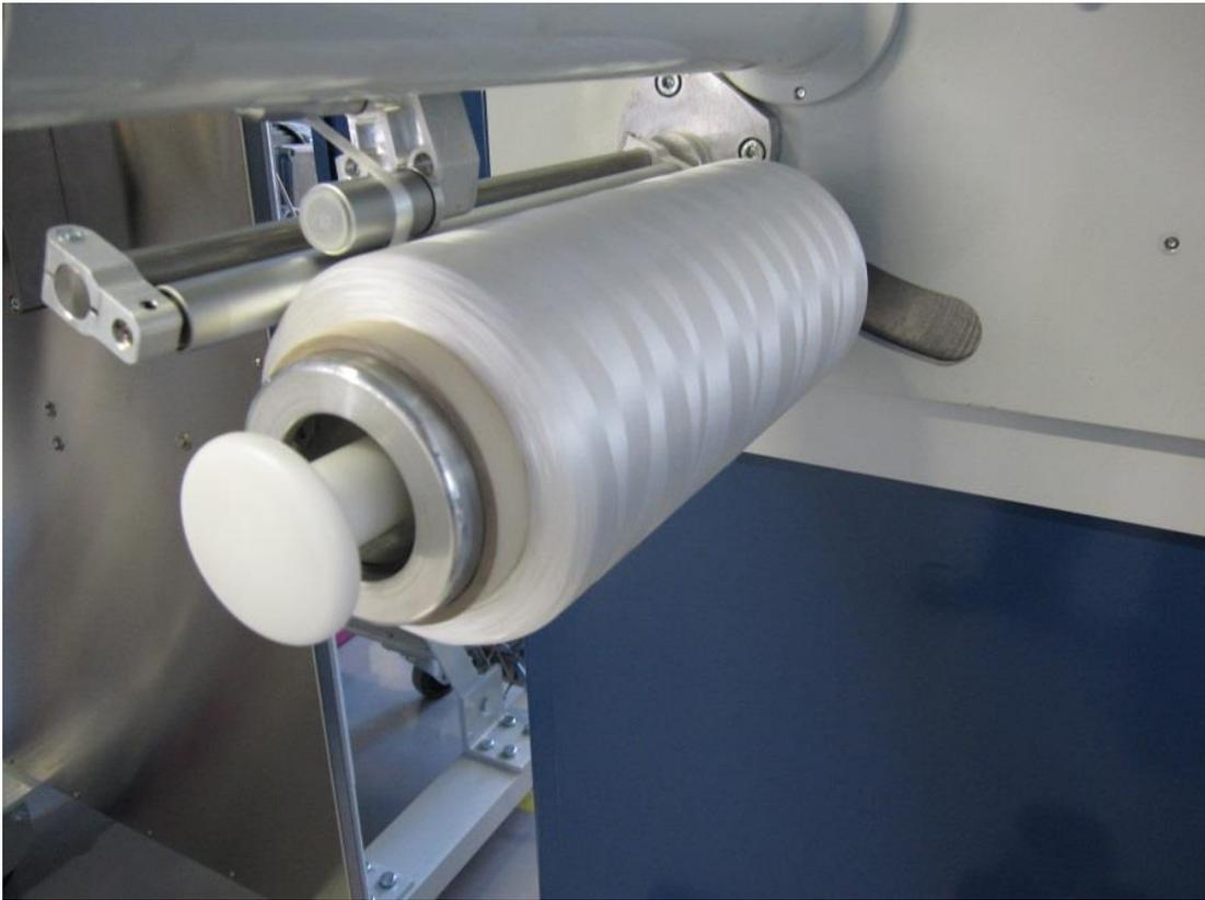
**Figure 3 Winding of 12K precursor fiber**
