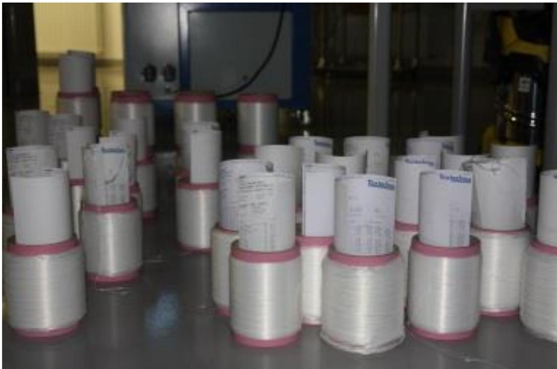
**Figure 4 Some of the PE precursor spools produced at the HPFC pilot line during NEWSPEC**
