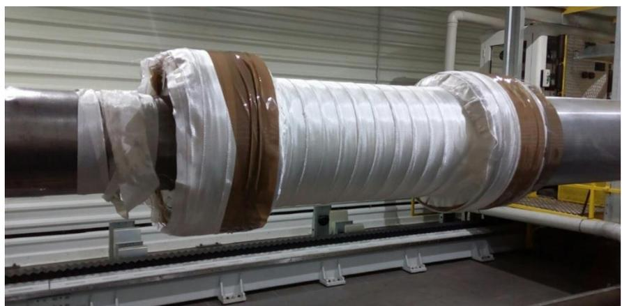
**Figure 21 (upper left) New functionalized CFs (upper right) Produced high pressure natural gas storage vessels and picture of semi-finished demonstrator on the mandrel with winded technological shell (bottom right).**
