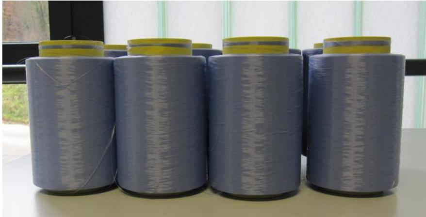
Figure 11 Mass spools with the produced bicomponent PE fibers
