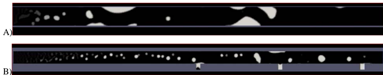
Figure 34: A snapshot from the simulation application showing bubbles (grey colour) and liquid (dark). In the top figure it is shown how gas bubbles accumulate on the superhydrophobic surface (initially all bubbles are small like on the left of the figure). In the bottom figure it is shown how adding valves remove the accumulated bubbles to the outside.
