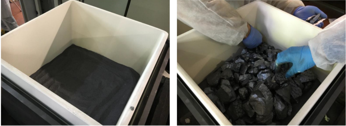
Figure 22: Charging of the crucible with 50% recycled material from GARBO on the bottom (left) and 50% new polycrystalline silicon from Wacker Chemie on the top (right)
