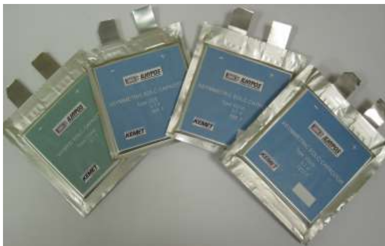
Figure 26. ILHYPOS hybrid and asymmetric prototypes with IL-based electrolyte.
