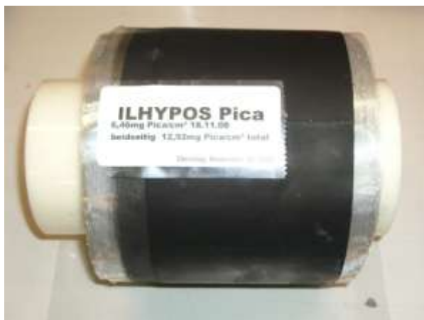
Figure 21. Coil of the final electrode processed on Al-expanded metal collector.
