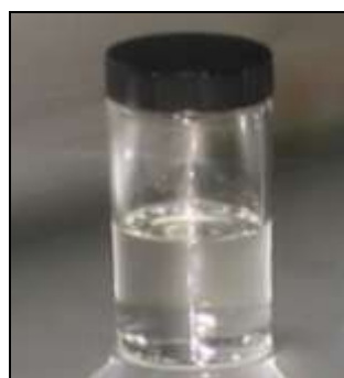
Figure 10. Photo of a \text{PYR}_{14}\text{TFSI} IL sample synthesized by ENEA.
