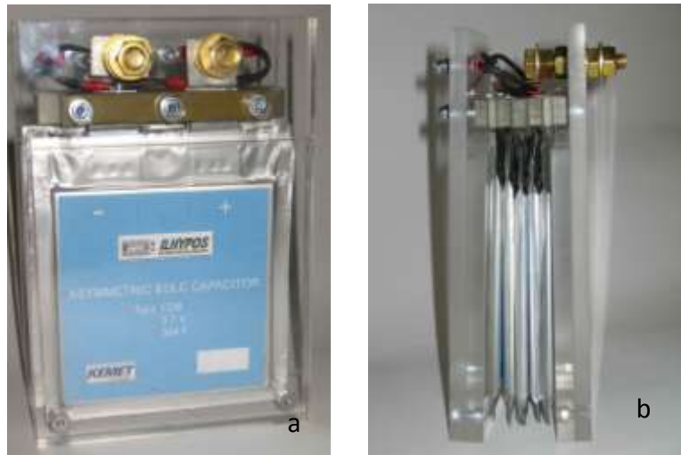
Figure 27. ILHYPOS prototype module with 5-cell in series: a) front view; b) side vie.
