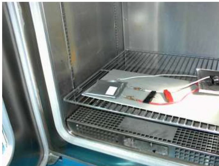
Figure 29. Symmetric SC prototype in a climatic chamber during test.
