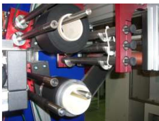
Figure 20. Assembling electrode materials and collector.
