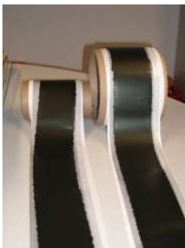
Figure 19. Coils of positive electrode.
