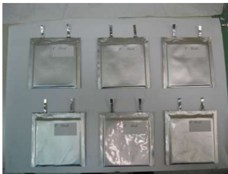
Figure 25. Complete set of ILHYPOS symmetric carbon/carbon prototypes with IL-based electrolyte.
