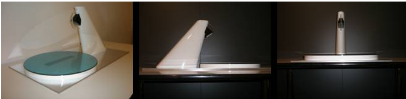
Figure 13: Real-size SATCOM antenna mock-up with inserted demonstrator array (see arrow in the left picture)
