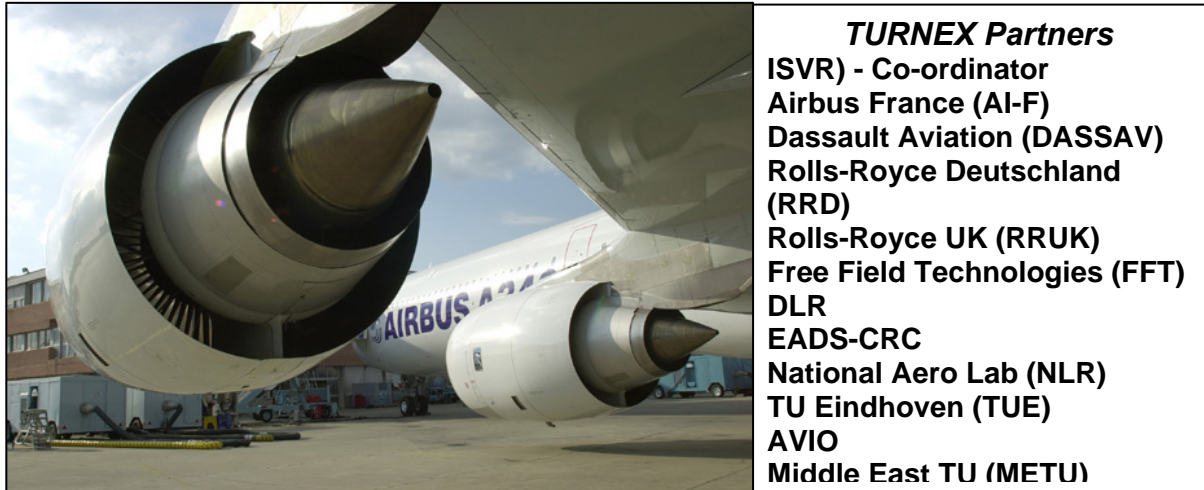
Figure 1.1: Bypass exhaust nozzle and the hot core exhaust nozzle of a Rolls-Royce Trent 500 on an Airbus A340 and TURNEX Consortium Partners
