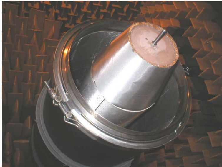
Figure 1.8: ISVR/RR No-flow rig with Inner & Outer Lined Bypass and Afterbody Liner Configuration
