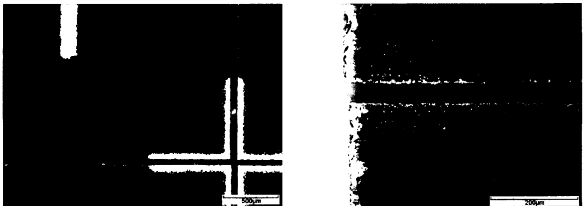
figure 8 A microscope image of a solarcell edge after trenching with the water-jet-guided laser shows that the bottom line is very regular and the kerf is clean.
