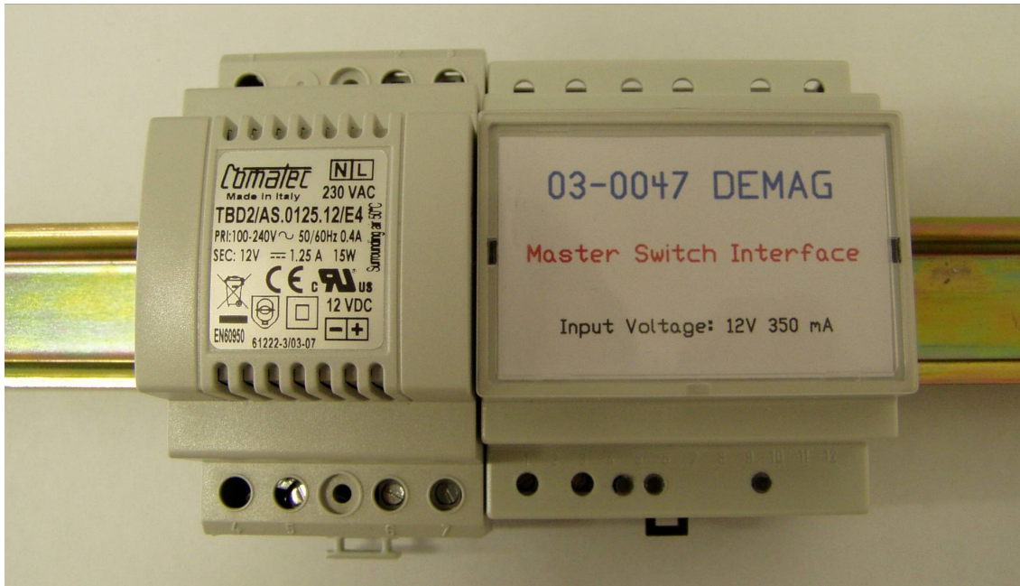
Figure 7: Overall view of the master switch unit (MSI + power supply)
