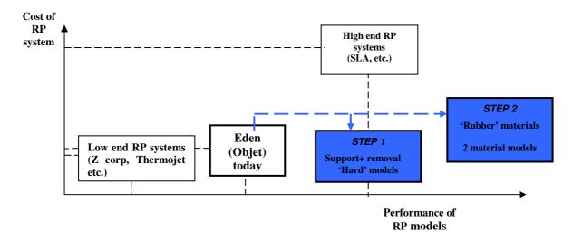
The aim is to have a high quality rapid prototyping system with more flexibility and functionality than the SLA-type of systems at the price of a concept modelling system or slightly higher.
