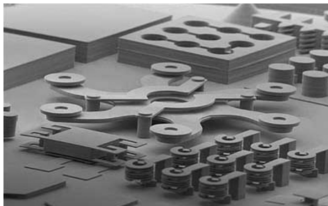
Figure 6: one of the first MEMS devices. At the bottom left with the C-shaped wings is an accelerometer.
