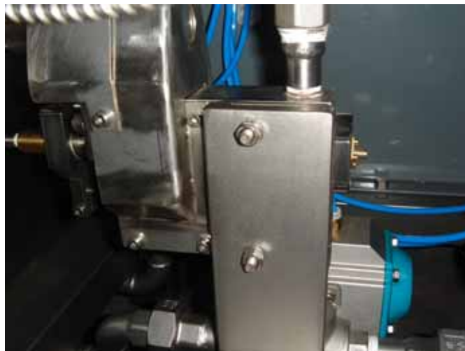
Figure 5 – Details of the EDY system: VOPS probes /2
