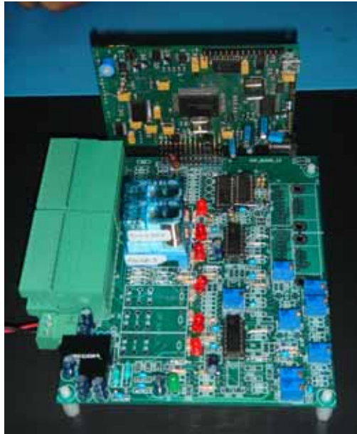
Figure 7 – Details of the EDY system: VOPS probes and control electronics /2
