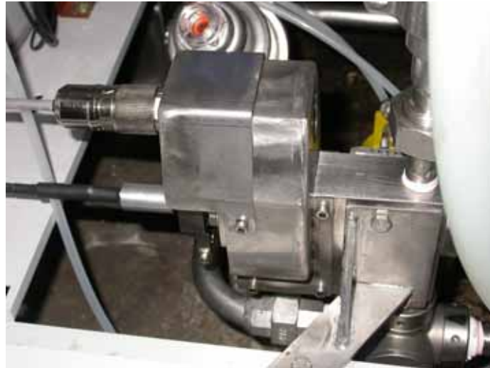
Figure 4 – Details of the EDY system: VOPS probes /1
