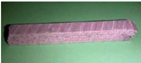
Cable stack with ceramic insulation
