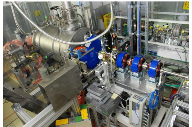
Figure 5: SRF photoinjector in the ELBE accelerator hall.
