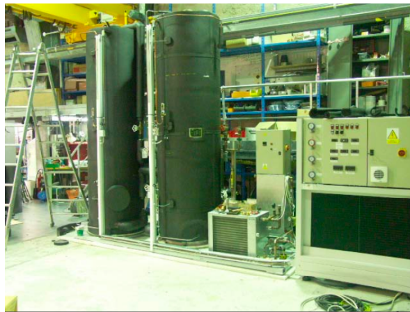
Figure 4 - Anti-radon factory at LSM, designed to provide 125 \text{ m}^3/\text{h} with a radon level of approximately 15 \text{ mBq}/\text{m}^3 .
