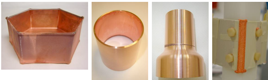
Figure 5 - Electroformed copper parts with different geometry and soldering assay obtained in the electroforming setup at the University of Zaragoza.
