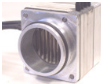
Figure A1.2 Prototype of the electrical air heater used at the inlet of the intake manifold of the engine.
