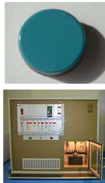
Figure 7. (a) Flame-sprayed glass coating on aluminium alloy substrate; (b) equipment for simulative wear testing of glass coated aluminium
