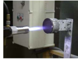
Figure 2. Depositing a glass coating by flame spraying
