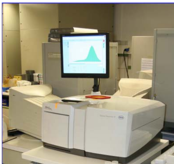
Roche GS FLX System (454) used at MPIMG #6 (~100 Mb per run, ~250 bp read length, ~400.000 reads)
