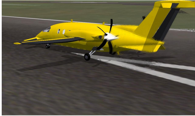
The flight simulator: Future-Wing aircraft within with the deformed left half-wing ( “aileron” down )
