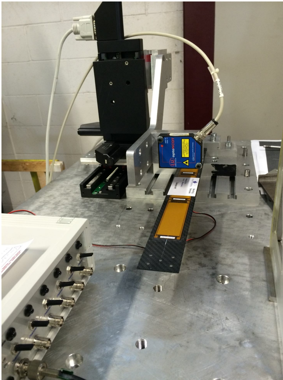
Test of a bending specimen: the high voltage six-channel amplifier is visible on the left of the figure
