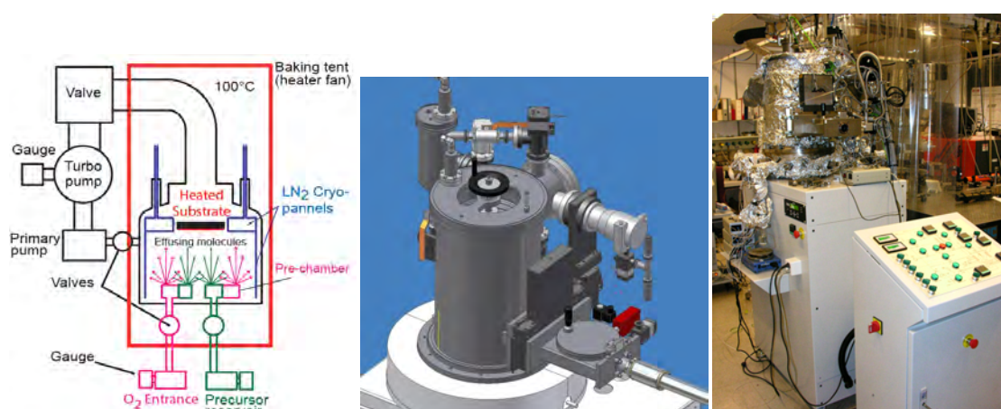
Figure 1: Schematic cross section through CBE process chamber (EPFL, left), CAD drawing of new reactor (ABCD, center), photograph of new reactor (ABCD, right).
