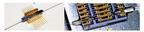
For us, the most interesting use of an SOA is to increase the output power of hybrid lasers in order to reach the specifications required for applications in various optical networks. First results with tunable lasers are very promising. Preliminary measurements suggest that, using an SOA at the output of a tunable laser, we will be able to couple 20 mW of output power to a fiber.
