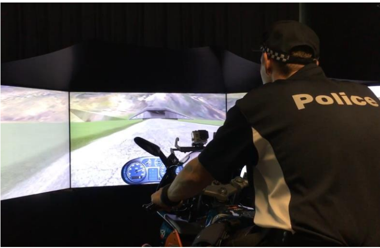
A participant rider during a test with the ABRAM simulator at MUARC.
