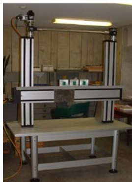
Figure 3-1: Mechanical scanner with three movable antennas
