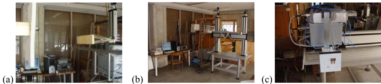
Figure 3-8: SAR imaging System with mechanical scanner
