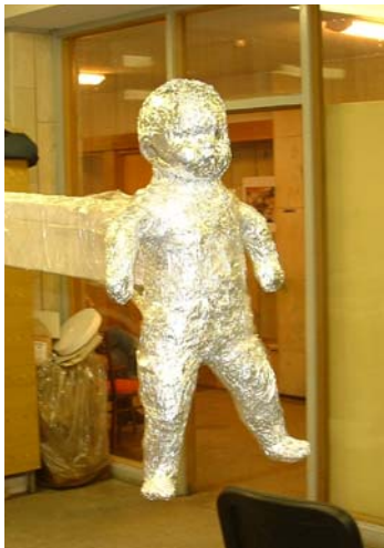
Figure 3-18: SAR imaging of a doll wrapped with metal foil in frequency band 3.1 – 10.6 GHz
