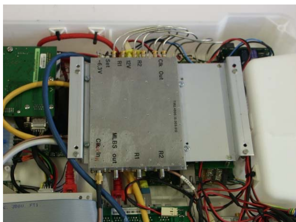
Figure 2-16: RF radar electronics
