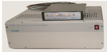
Figure 3-3: Two-channel sampling converter with sampling unit
