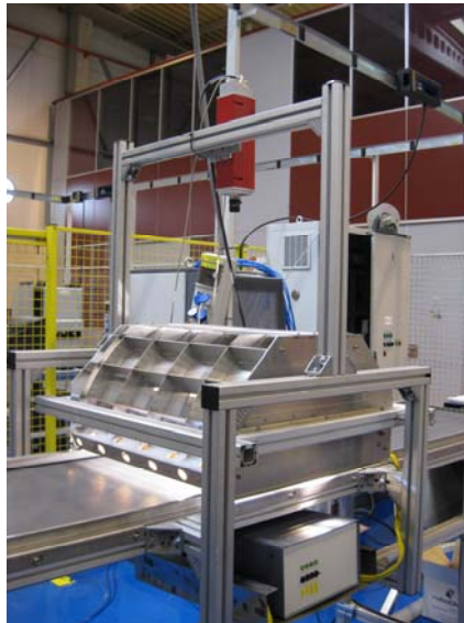
Fig. 2.13. Integrated vision module: power supply, light and camera
