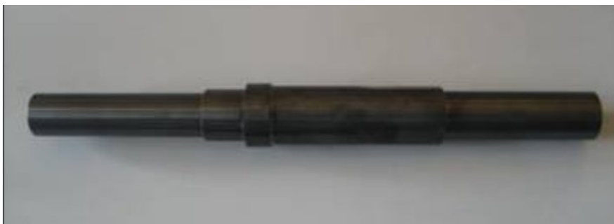
Figure 1-2: Piston with chromising - DLC
