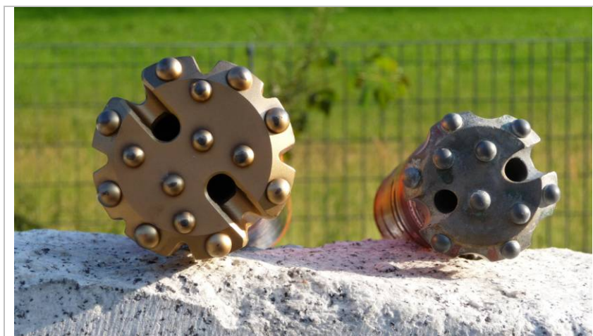
Figure 3-20: Comparison between 3 1/4 and 2 1/4 inches STREAM hammer prototypes
