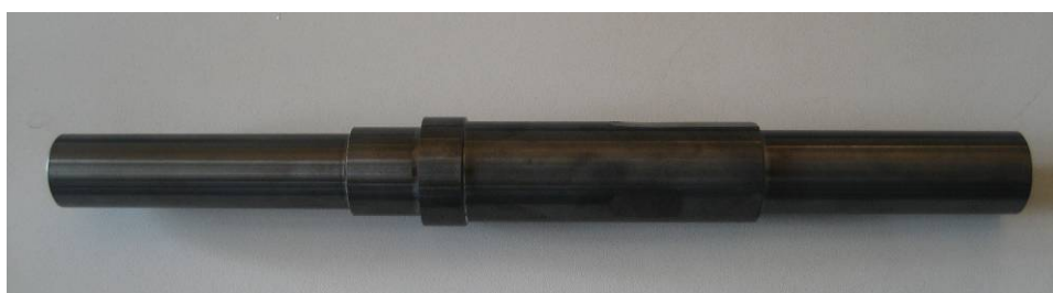
Figure 3-7: Piston with chromising – DLC
