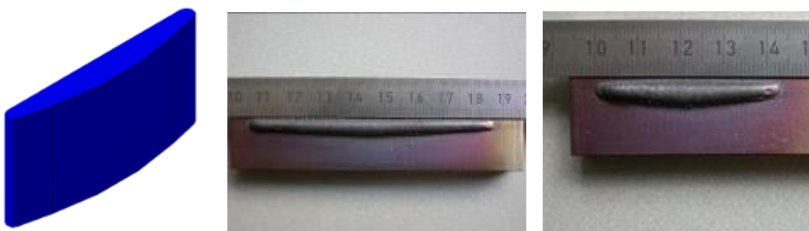
Figure 26. Left: digital drawing of Banana shape. Middle: produced piece sample 4 of 80mm length, Right: produced sample 5 of 40mm length shape.
