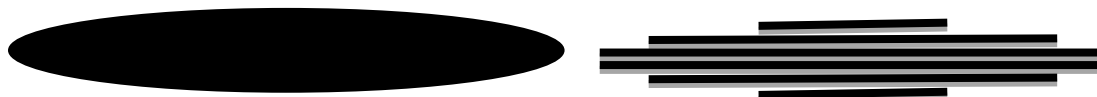
Figure 1. : Left: production of a track using variable track width programming, right: production of the same geometry using multiple passes. The profit of the former in terms of production time is obvious.
