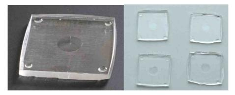
Roughness values  $R_a$  for all measured lenses were close to 0.018. This was higher than  $R_a$
