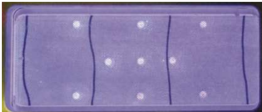
Fig. 1: L4CW-Demo quartz-glass sub-unit showing energy optimal, homogeneous irradiation
