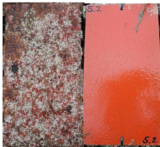
Fig 14. (Left) Photographs of panels (Control and LEAF 5.2 formulation) exposed in Sweden (Right) Photographs of panels (Control and LEAF 5.2 formulation) exposed in Sweden. The control formulation contains the same components as in LEAF 5.2 but without the biocides.
