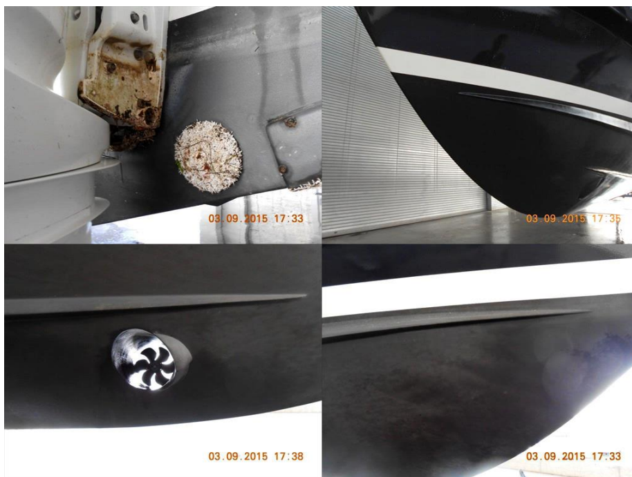
Fig 17. Example of boat hull after completed test for 4 months. No visible fouling can be observed, except on the circular cathodic protection area which had not been painted with LEAF paint.
