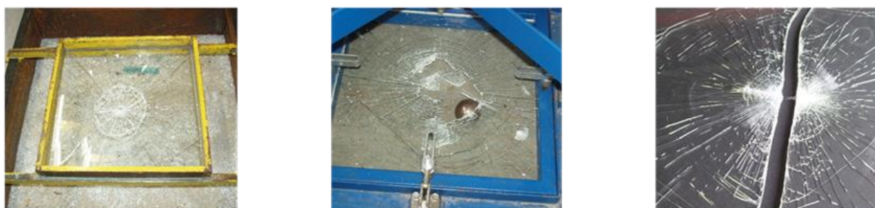
Figure 2.-2.: Results of ball drop testing for 3 different glazing variants with (from left to right): PVB-28% softener; PVB-GF21% softener; softener-free PVB.
