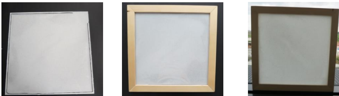
Figure 2.2-3.: PCM-Demonstrators 0.25 m² arera, without and with wooden frames.
