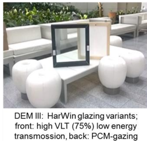
Figure 2.: HarWin Demonstrator glazing variants and windows with glazing 500x500 mm 2
